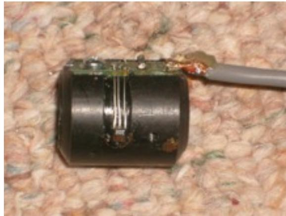
Board with cable and Hall sensor mounted off the side of PC board Note surface mount capacitor ( Yellow cube) Note: pc board chage to single mount hole.
