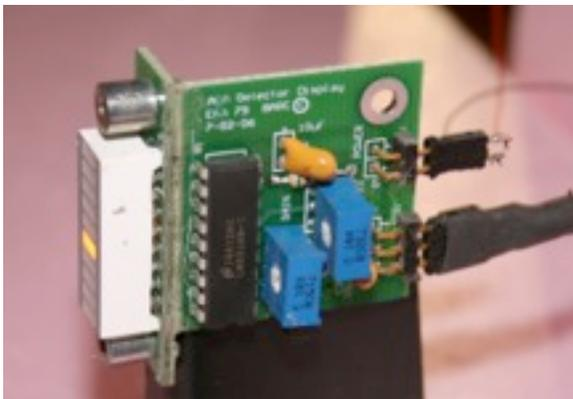
The AOA display board requires minimal panel space, but should be mounted high on the panel to stay within your peripheral field of vision while looking outside.
