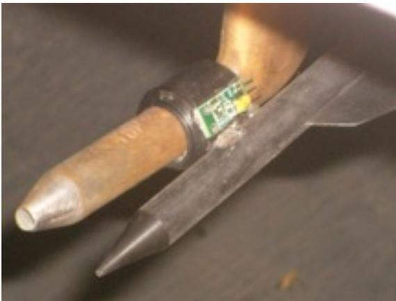
**AOA Vane Mounted next to Pitot tube** (prototype) lock with 4-40 set screw.
